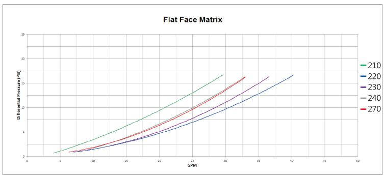
Flow chart shown as a sample curve. Actual flow and pressures will vary depending on fluid used. Chart data for Viscor 1487 Calibration Fluid at 72°F.
